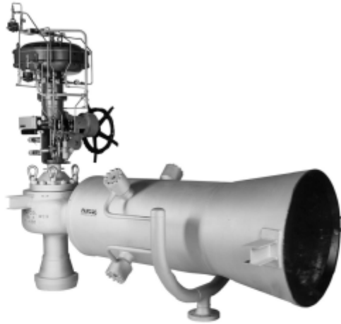
1-9445 Limiphon reducing/desuperheating valve supplied with angle body, bottom inlet and injection chamber provided with multiple LVM type spring nozzles welded downstream.
