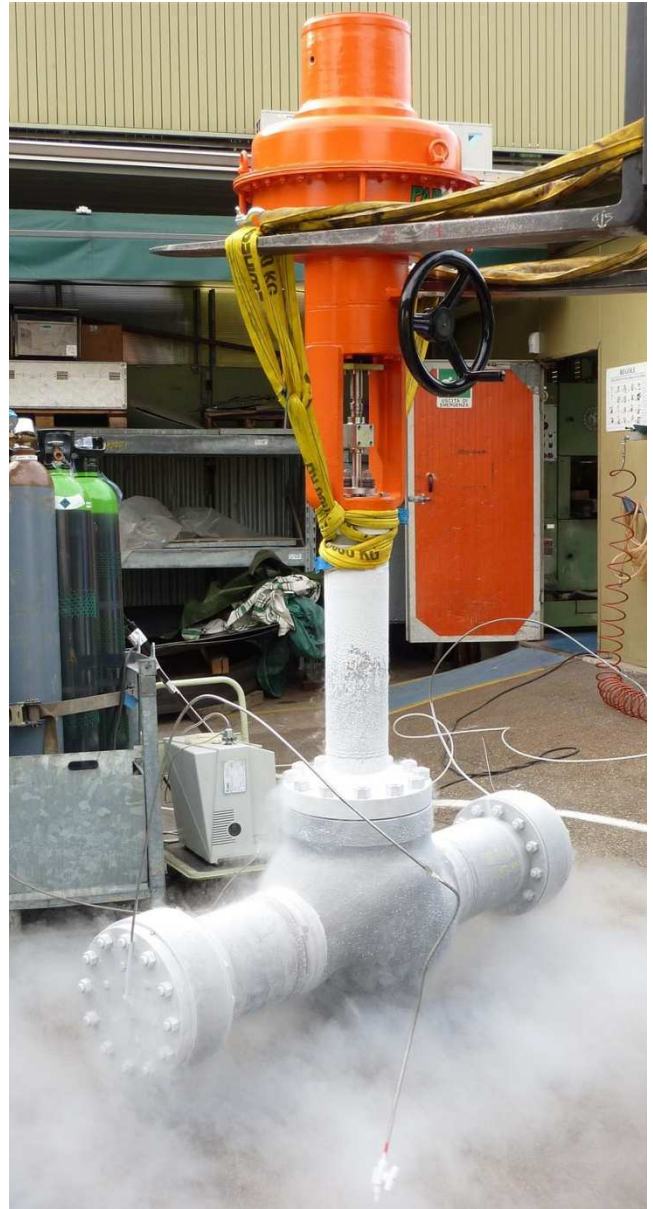
VEGA CRYO CONTROL VALVE AFTER TYPE TEST ON LIQUID NITROGEN
