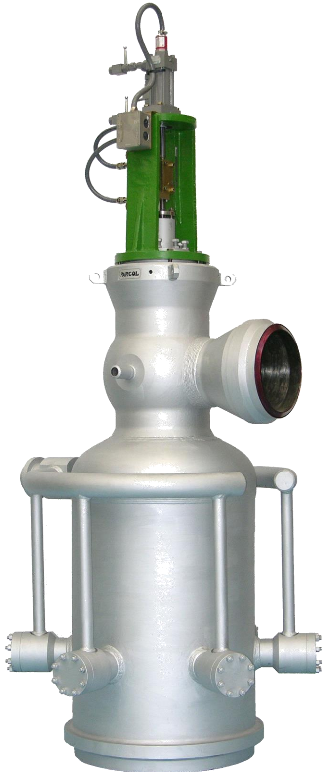
Parcol 1-5745 designed for by-pass service in hypercritical boiler power plant with upstream steam temperature 612°C and upstream pressure 75 bar.
